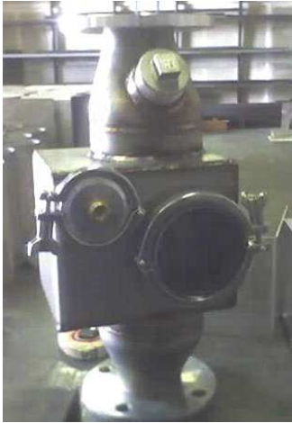
A Vent Monitor, which maintains a low breaking pressure water seal within vent pipes, yet allows prevention of vacuum lock within the system.
